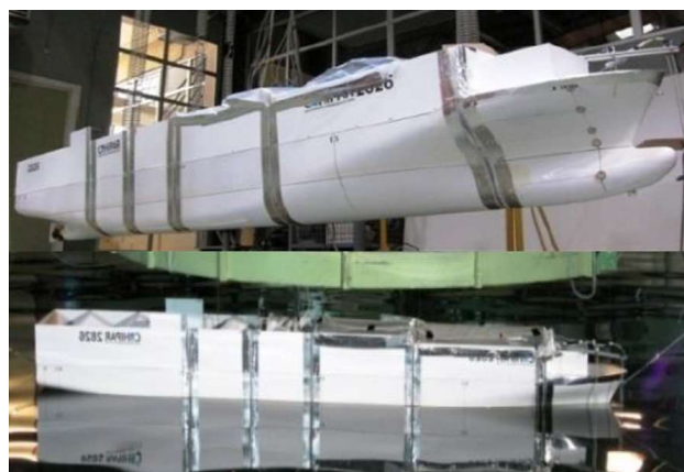
Figure 0-16 Hydroelasticity test of a segmented model of 10,000 TEU containership
