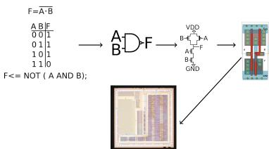
Designing digital circuits is mapping logical functions to transistor level equivalents, *implemented* on a chosen platform, ASIC or FPGA.
