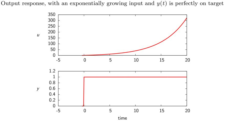
We are capable of achieving perfect tracking in y(t) by using applying an optimal u(t)
