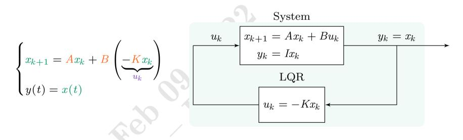
The stability of the closed-loop is determined by the eigenvalues of matrix  $A_{\rm CL}$ The closed-loop dynamics,
