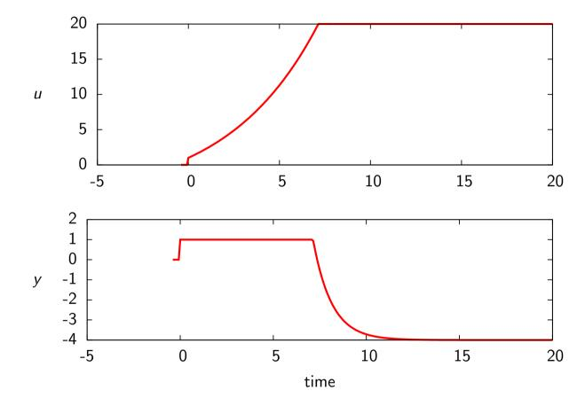
The saturation of the input at the constraint destroys the perfect output response y(t)
