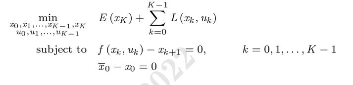
The controls  $\{u_k\}_{k=0}^{K-1}$  are the true decision variables of the optimisation The state variables can be eliminated by forward simulation
