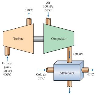
The turbocharger of an internal combustion engine consisting of a turbine, a compressor, and an aftercooler is considered. The temperature of the air at the compressor outlet and the minimum flow rate of ambient air are to be determined. Assumptions: 1 All processes are steady since there is no change with time.
