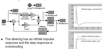
. The guidance proposed by the Controller cannot be effectively implemented and, as the distance of the rocket approaches the desired value, it will pass and overshoot
