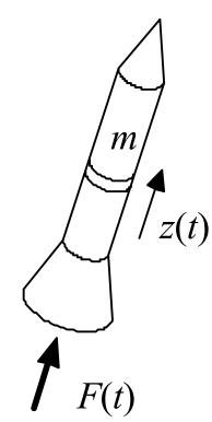
• The controller has two parallel functions, the first of which follows the magnitude of the deviation (the difference) and multiplies it by a constant of 30 and the other with the slope of deviation (i.e. the differential derivative) and multiplies it by 31. Total control, i.e. the force required (u(t) = F(t)) is calculated as the sum of these two control forces.
