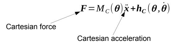
Cartesian dynamics parameters can be calculated using joint space dynamics + Jacobian. E.g.
