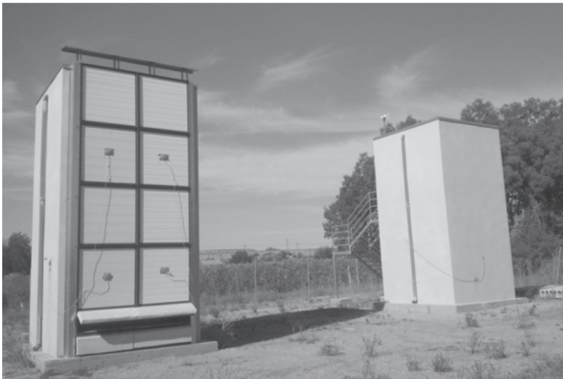
Figure 23.12 Experimental set-up to test a ventilated façade with macro-encapsulated PCM in its air cavity located in Spain (de Gracia et al. , 2013a).
