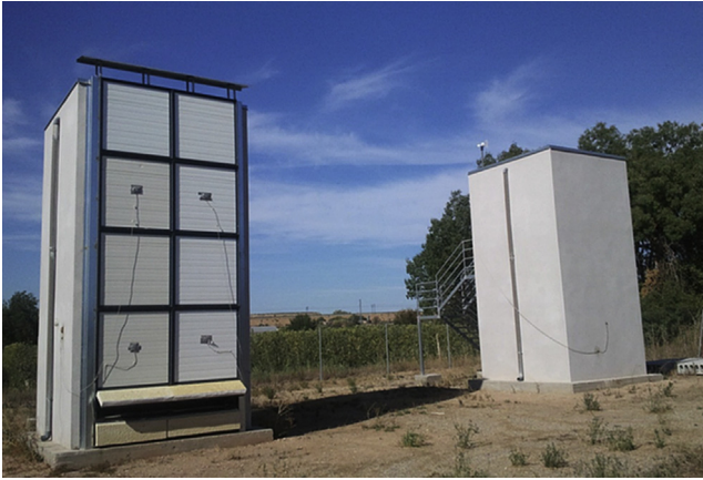
Figure 7.19 Experimental setup to test a ventilated façade with macroencapsulated PCMs in its air cavity located in Spain (de Gracia et al., 2013a).
