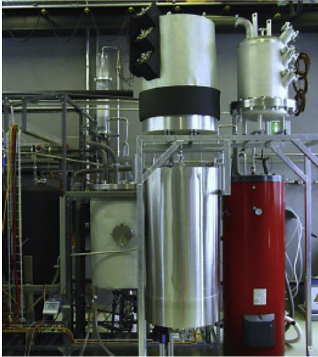
Figure 7.20 Double-stage NaOH/H 2 O prototype built at the Swiss Federal Laboratories for Materials Science and Technology (EMPA) (Weber and Dorer, 2008).
