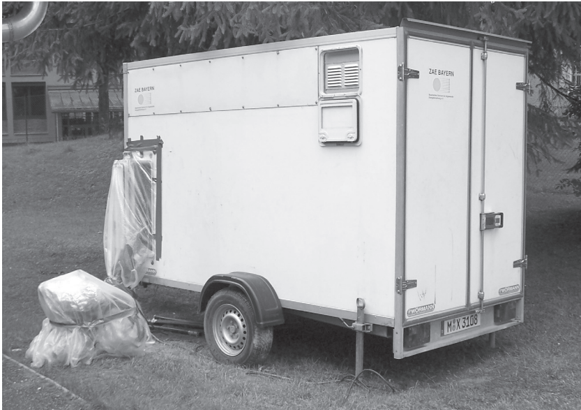
Figure 6.5 Trailer with Thermal Response Test equipment connected to a test borehole.
