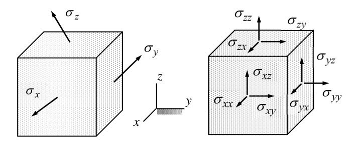
The first index of a stress component refers to the direction of the surface normal and the second that of the force component.
