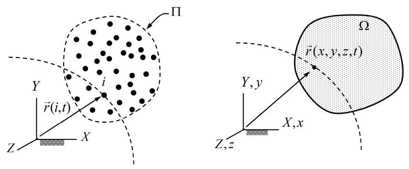
Time can be considered as the curve parameter for the particle paths. In stationary description, one considers only the initial position  $\Omega^{\circ}$  (at t=0 say) and the final position  $\Omega^{\circ}$  (at some other instant of time) and the curve parameter can be omitted.
