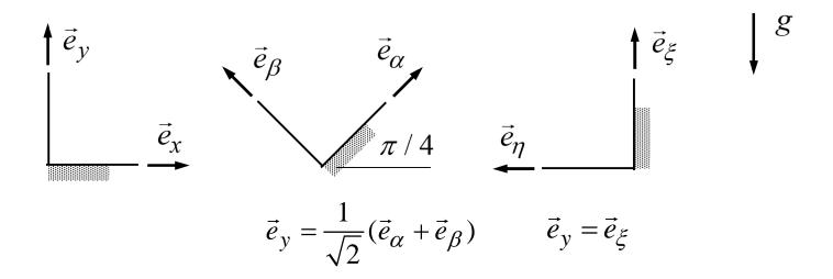
**EXAMPLE** Second order tensor  $\vec{a}$  can be represented in any coordinate systems of the figure starting with the known representation  $\vec{a} = a\vec{e}_y\vec{e}_y$  in the Cartesian system. Using the relationship between the basis vectors
