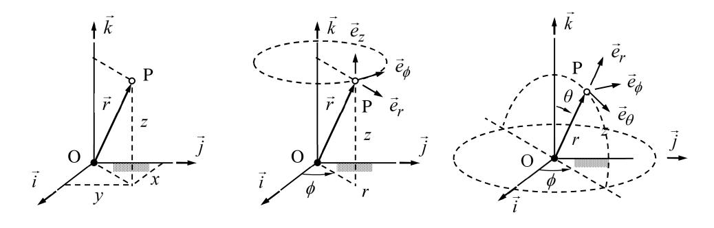
Transformation from one coordinate system to another requires the relationship between the basis vectors. Considering  $\vec{a}$  of a planar case and using the relationship between the basis vectors of the Cartesian and polar coordinate systems shown ( $c \sim \cos$ ,  $s \sim \sin$ )
