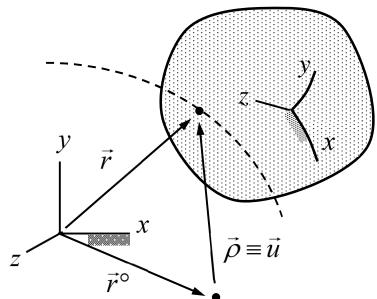
Displacement  $\vec{u}(x, y, z)$  is the primary unknown of a linear elasticity problem and other quantities like strain and stress are (finally) expressed in terms of it.
