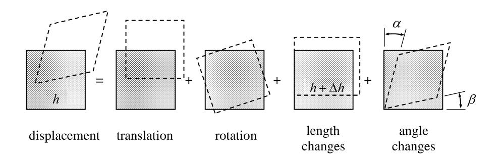
The geometry is described altogether by 12 parameters, of which 6 define the rigid body motion and remaining 6 the deformation (normal and shear components).
