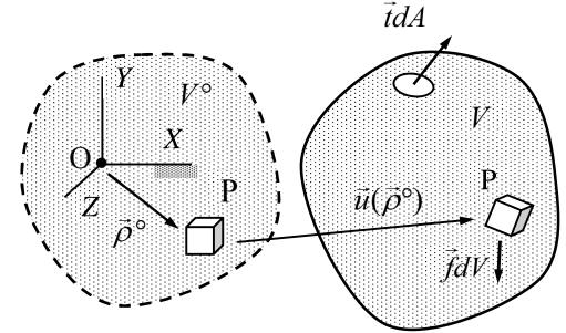
Assuming an equilibrium setting (geometry, stress, loading etc.) the local forms can be used used to find a new equilibrium setting (actually displacements of the particles) when, e.g., external given forces are changed in some manner.
