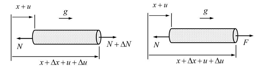
The cases where the material element is inside the bar and at the right end differ.
