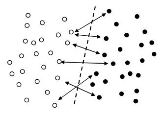
The ratio  $\Delta \vec{F}/\Delta A$  of the interaction force resultant  $\Delta \vec{F}$  to the area of the interaction  $\Delta A$  is assumed to be constant  $\vec{\sigma}$ , when the area *is not too small nor too large*, therefore also  $\Delta \vec{F} = \vec{\sigma} \Delta A$ . Although a certain range of lower and upper limits is involved, continuum mechanics uses the relationship in form  $d\vec{F} = \vec{\sigma} dA$ .
