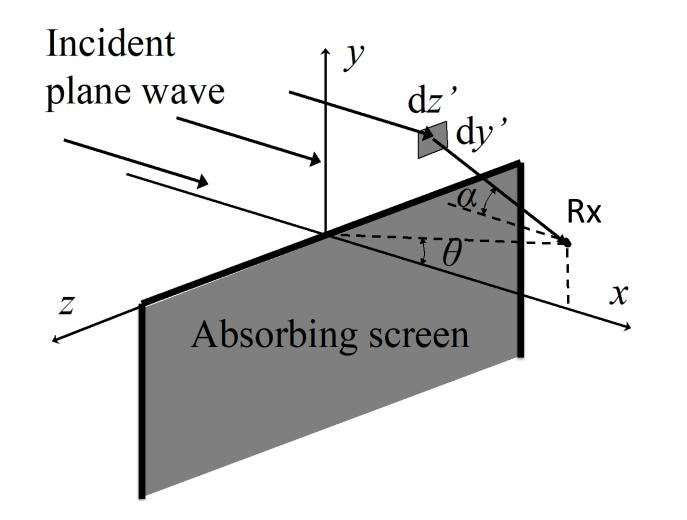
Q3: A tip of the absorbing screen is just the heights of the transmit and receive antennas, i.e., h = 0. What is the loss of the link, compared to an unobstructed link?
