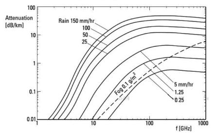
Figure 10.3 Attenuation due to rain and fog.
