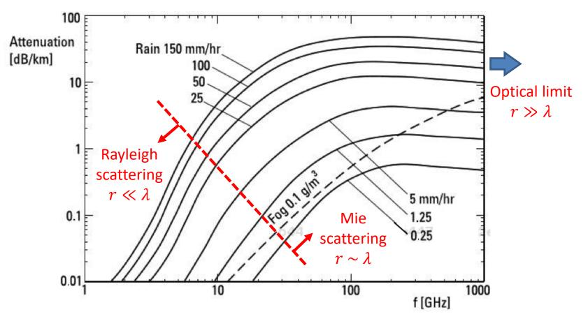
Figure 10.3 Attenuation due to rain and fog.
