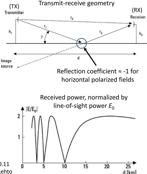
Q5: There are line-of-sight and groundreflected waves, with a reflection coefficient of the ground -1. Which of the following leads to very small power at the receiver?
