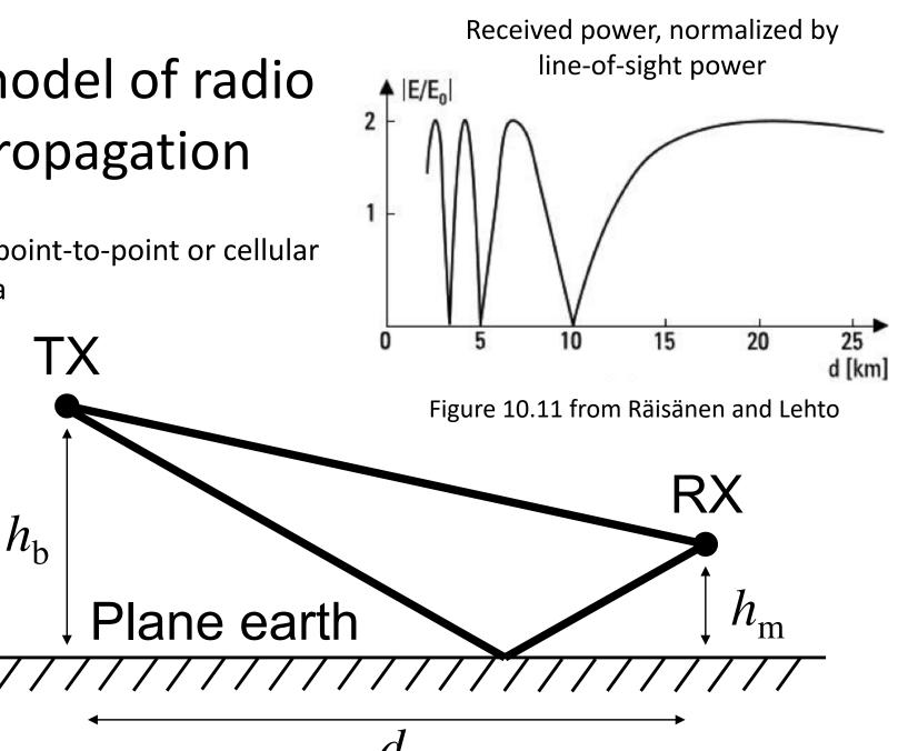
Q4: There are line-of-sight and groundreflected waves, with a reflection coefficient of the ground -1. Which of the following is <u>incorrect</u> explanation?
