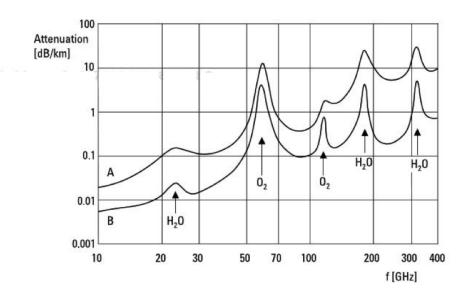
Figure 10.2 Attenuation in clear atmosphere versus frequency. Curve A: at sea level  $(T = 20^{\circ}C, \text{ water vapor density 7.5 g/m}^3)$ . Curve B: at altitude of 4 km  $(T = 0^{\circ}C, \text{ water vapor density 1 g/m}^3)$ .
