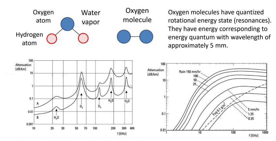
Figure 10.2 Attenuation in clear atmosphere versus frequency. Curve A: at sea level Figure 10.3 Attenuation due to rain and fog.  $(T = 20^{\circ}C, \text{ water vapor density 7.5 g/m}^3)$ . Curve B: at altitude of 4 km  $(T = 0^{\circ}C, \text{ water vapor density 1 g/m}^3)$ .
