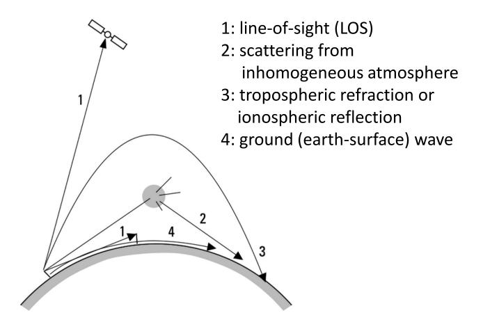
**Figure 10.1** Propagation mechanisms of radio waves (numbers refer to different mechanisms described in text).
