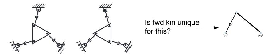
Different type of singularity compared to serial mechanisms. But in which way?
