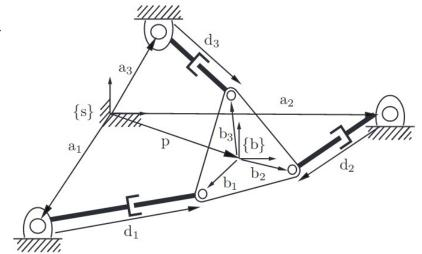
$$d_{i}^{2} = (p_{x} + b_{ix}\cos\phi - b_{iy}\sin\phi - a_{ix})^{2} + (p_{y} + b_{ix}\sin\phi + b_{iy}\cos\phi - a_{iy})^{2}$$
