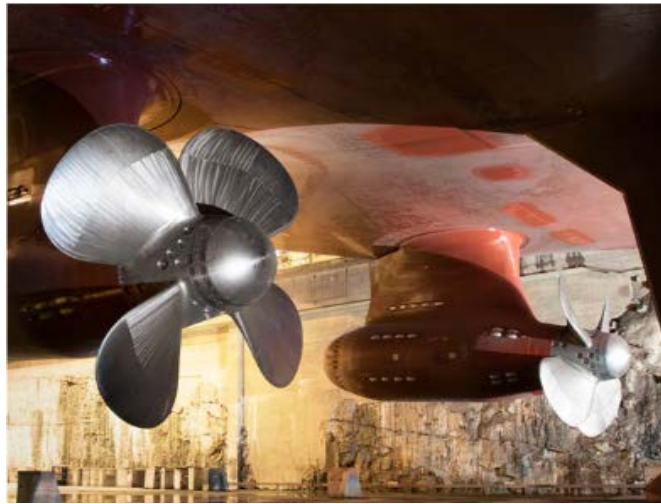
Figure 1.4 ABB Azipod VI system installed on a ship.
