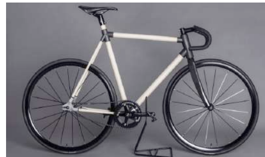
Light and durable nanocellulose tubes by Tiina Härkäsalmi. Bicycle by Kim-Niklas Antin & team. DWoC project 2017, photo Eeva Suorlahti
