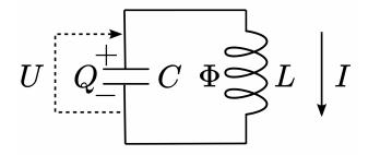
From the above circuit figure, we also see that the voltage drop across the inductor is U; hence, from Lenz's law we have  $\dot{\Phi} = U$ . Therefore,
