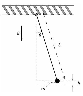
We consider a pendulum of length  $\ell$  and mass m that subtends an angle  $\theta$  with respect to the center.
