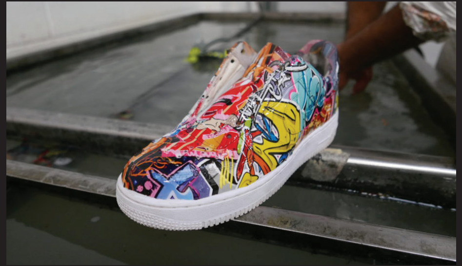
“water transfer” eli “hydrographic dipping” menetelmä
