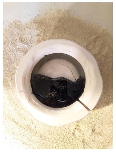
A multiple layer, hand-built mold allows for the individual mold layers to crack without the crack going all the way to the glass layer. It also saves a considerable amount of material, and allows for faster and more even cooling of the glass after the casting process.
