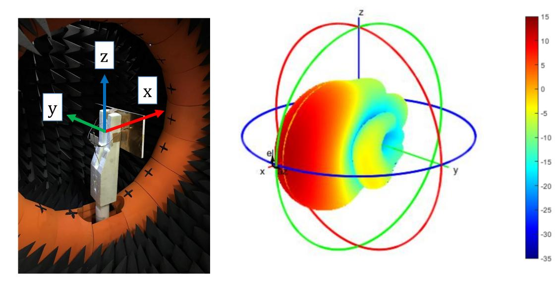
AUT (3 x 1 patch array): two principal pattern cuts as total realized gain (dBi) are presented in polar cuts of the standard spherical coordinates system
