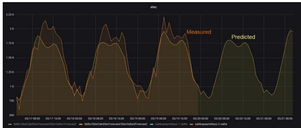
Figure 21: Example view of online energy prediction model for Sello in Action E6-1. This is a short term view (2 days prediction for electricity demand for 1 electricity metering point. Source: VTT
