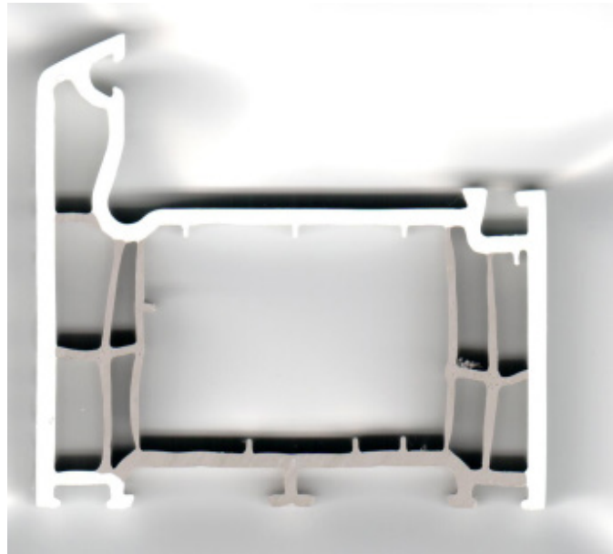
Figure 23. Window profile system with recycled content due to the incorporation of recycled material into the profile core
