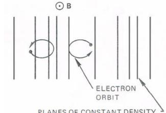
$$\rightarrow \omega^2 = \omega_p^2 + \Omega_e^2 \equiv \omega_h^2$$
