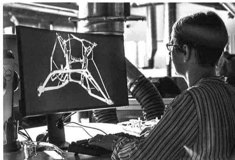
FIGURE 1.9 Autodesk DreamCatcher is a generative design system based on structural optimisation.
