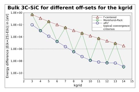
Figure 4.6: The k-grid was tested with respect to the grid density and the shift of the grid in reciprocal space. The shifts are defined in Eqn. (4.1).
