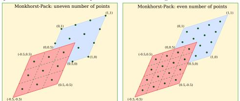
Figure 4.3: The Monkhorst Pack grid [162] in two dimensions for even and uneven numbers of grid points. In the left picture (uneven number of grid points) the  $\Gamma$  point is included in the grid.
