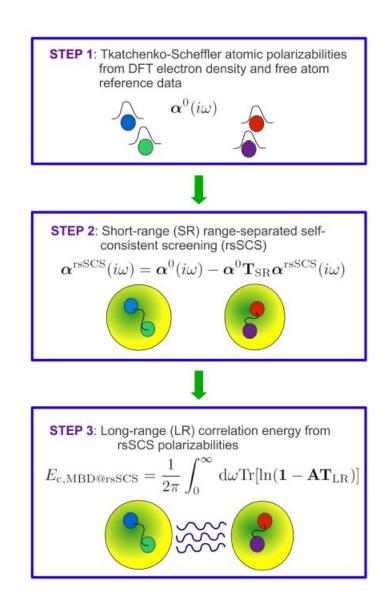
Figure 3.5: Schematic description of the MBD@rsSCS method.
