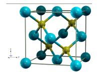
Figure 4.5: The crystal structure of silicon carbide in its cubic zinc blende structure (3C-SiC)
