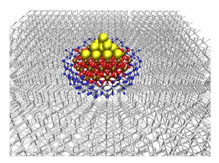
Figure 3.3: Example for QM/MM setup:  $Au_n@TiO_2$ . The adsorbed cluster and direct substrate vicinity defines the QM-region. The far field surrounding (grey particles) pictures a monopole field with formal charges (4+ for Ti and 2- for O). In the blue region, oxygen particles are still represented as monopoles, however Ti-cations are described with ionic pseudopotentials.
