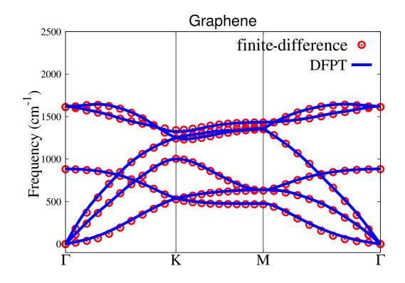
Figure 3.9: Vibrational band structure of graphene computed at the LDA level using both DFPT (solid blue line) and finite differences (red open circles). All calculations have been performed using a  $11 \times 11 \times 1$  k-grid sampling for the primitive Brillouin zone, tight settings for the integration, and a tier 1 basis set.
