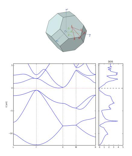
Figure 4.8: Band structure and density of states of the bulk Si test case as generated by the aimsplot.py script, which is located in the "utilities" directory. A schematic visualization of the Brillouin zone of the fcc Bravais lattice including some high-symmetry k-points is also shown (taken from Wikipedia).
