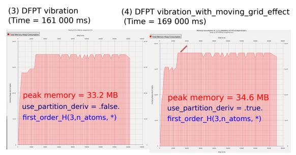
Figure 3.8: The memory profiles using valgrind are shown for DFT and three DFPT vibration keywords. It is clearly shown that the DFPT\_vibration\_reduce\_memory(28.4 MB) code just use nearly the same memory as DFT (28.0MB) calculation, while DFPT\_vibration(33.2 MB) and DFPT\_vibration\_with\_moving\_gird(34.6 MB) need higher memory because they stored matrix as (3,n\_atoms, \*).
