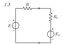
A battery, with an open-circuit voltage  $E_{\rm a}$  and internal resistance  $R_{\rm s}$ , is charged by a voltage source E through resistance R as shown in the figure. By using Kirchoff's laws, Ohm's law and the expression of power seen in the lecture, determine R so that the power flowing into the voltage source of the battery is  $P_{E_{\rm a}}$ .
