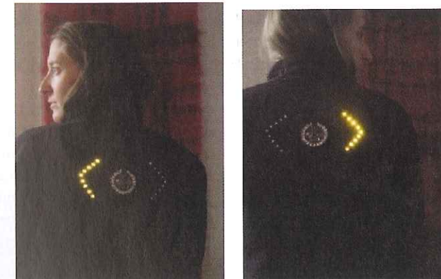
Figure 1.3 Turn signal biking jacket using e-textiles developed by Leah Beuchley
