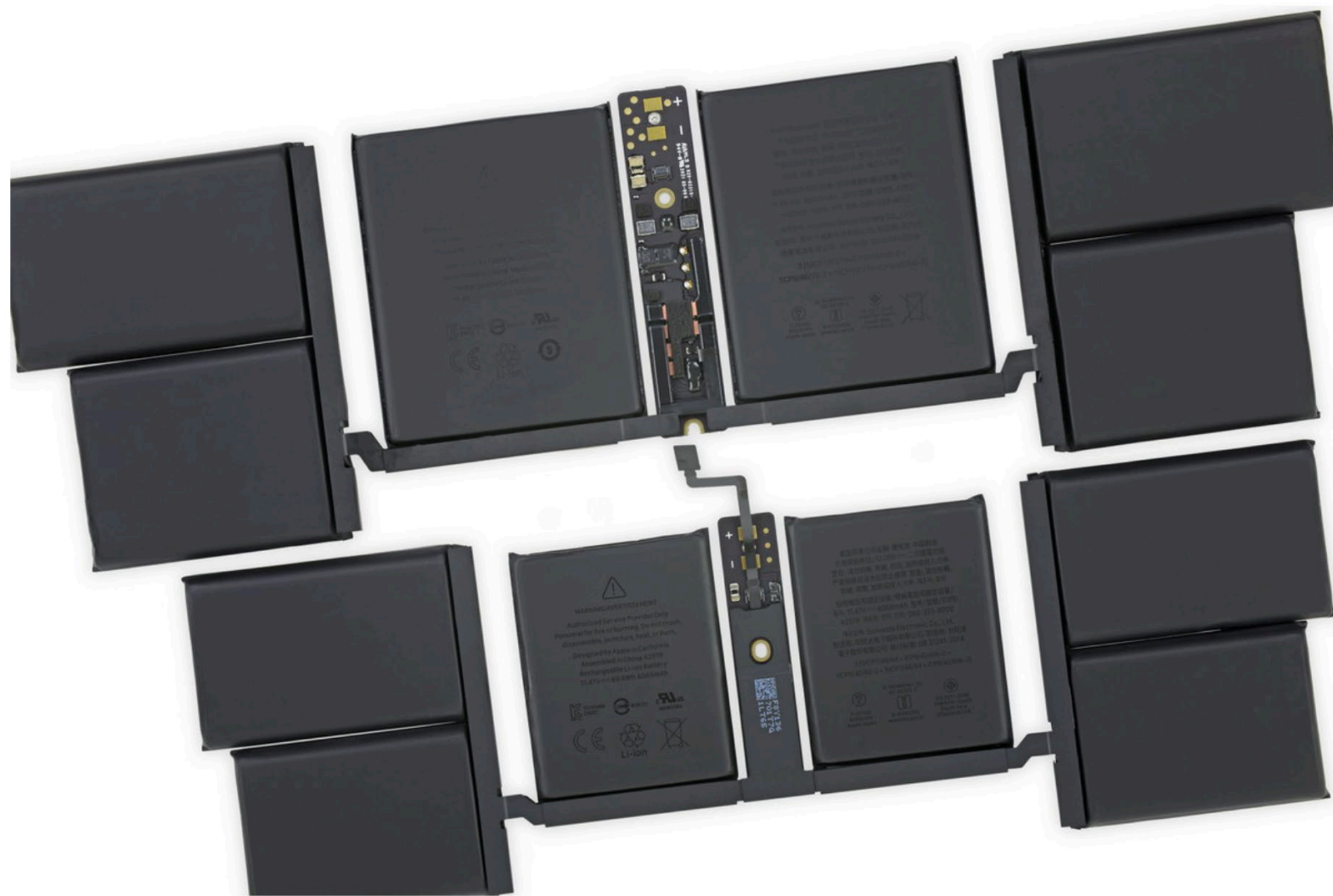
Batteries from the 16" (top) and 14" (bottom) 2021 MacBook Pros. Click to enlarge
