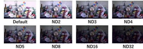
Fig.10 Effect of electrical ND filter sensitivity of OPF (photoelectric conversion efficiency)
