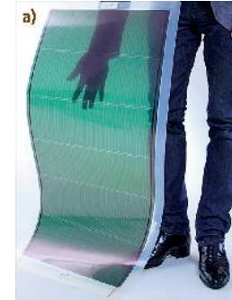
Commercial flexible see-through organic solar cell module. (Mitsubishi Chemical Corporation)
