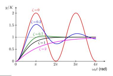
Step responses can be easily plotted using numerical simulation tools. If needed, an analytical solution could be obtained using the inverse Laplace transformation.
