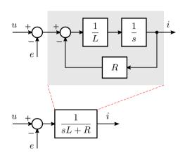
In the Laplace domain,  $s=\sigma+\mathrm{j}\omega$  is a complex variable. However, the differential operator and the Laplace variable can be used interchangeably in many cases.
