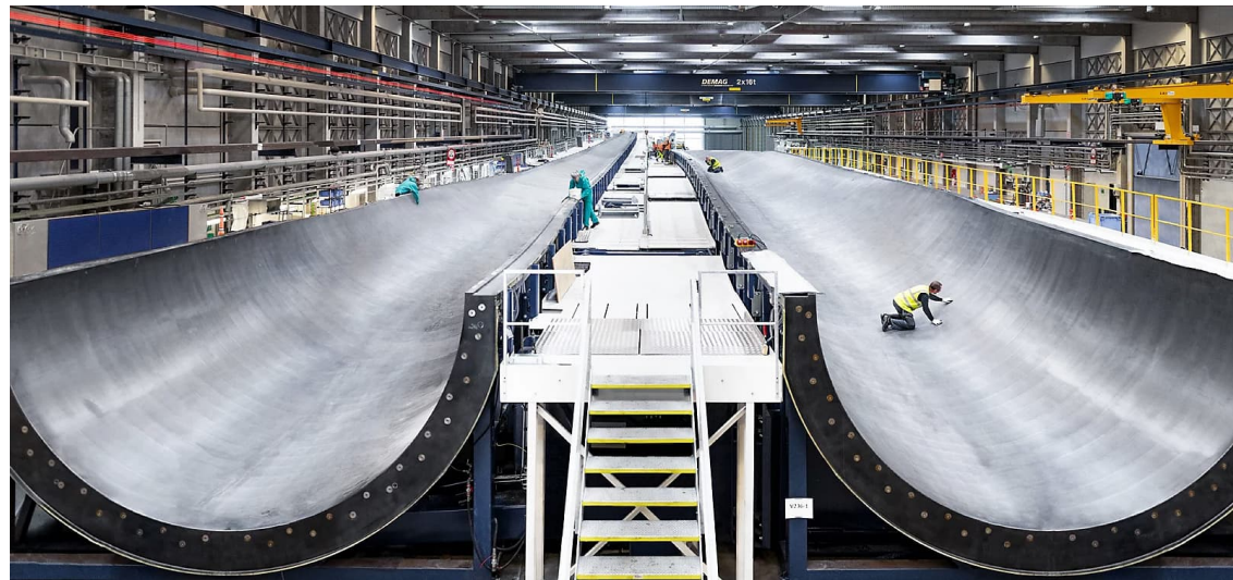
Manufacturing a blade for Vestas V236 wind turbine prototype Blade length 115.5m.
