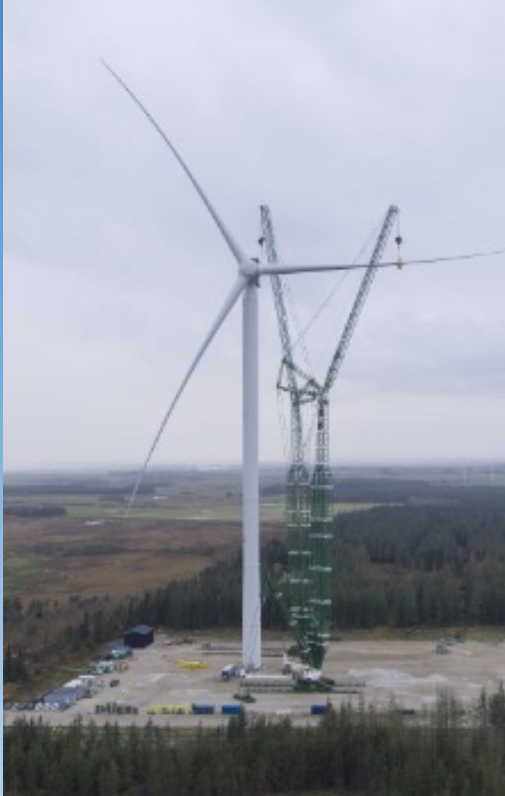
Siemens Gamesa's SG 14-222 DD prototype offshore wind turbine installed at the test centre in Østerild, Denmark Source : offshorewind.biz Dec 10, 2021
