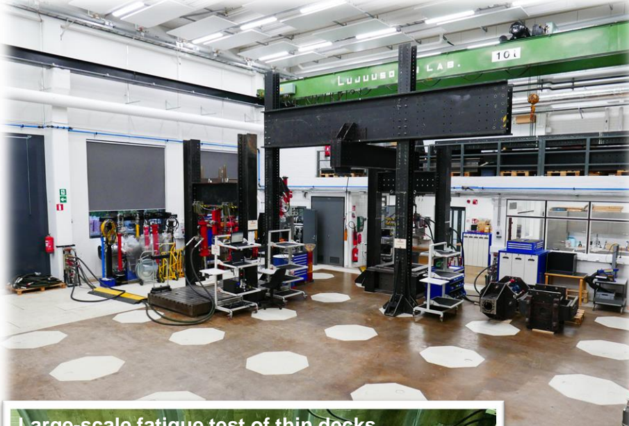
Large-scale fatigue test of thin decks
