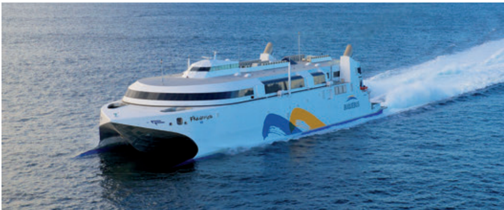
FRANCISO is the first dual fuelled fast ferry to operate with LNG as the primary fuel
