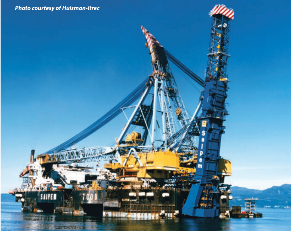
Semi-submersible crane and pipe lay vessel SAIPEM 7000 with J-lay tower
