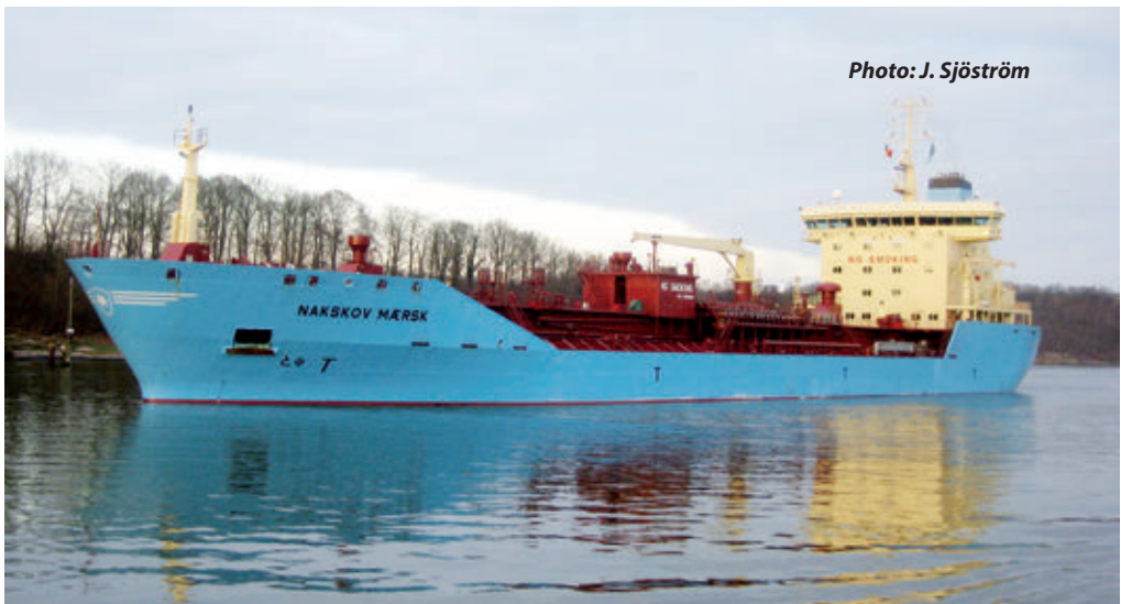
16 600dwt product carrier NAKSKOV MAERSK LBP = 133.0\text{m} , B = 23.4\text{m} , d = 8.40\text{m}
