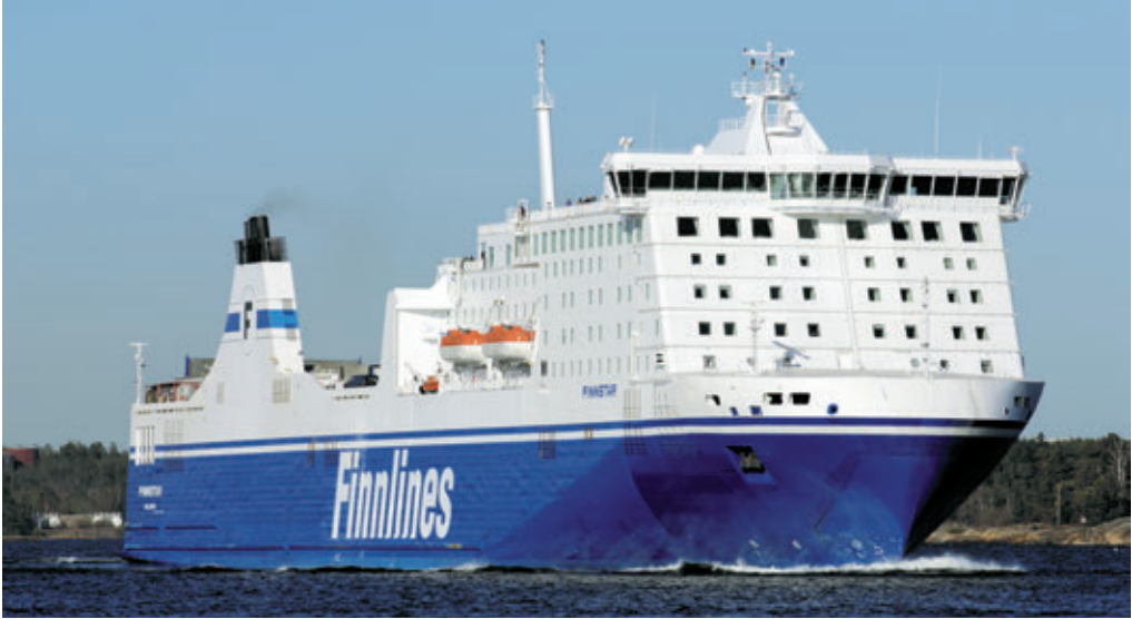
The Italian built giant RoPax ferry FINNSTAR for Helsinki/Travemuende link, 4200 lane metres, amenities provided for up to 500 passengers
