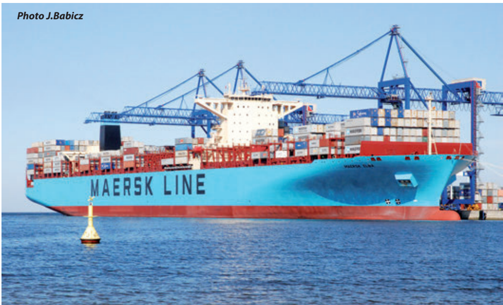
13,100TEU vessel MAERSK ELBA “Two islands” concept with accommodation separated from the engine room is characteristic for mega container ships
