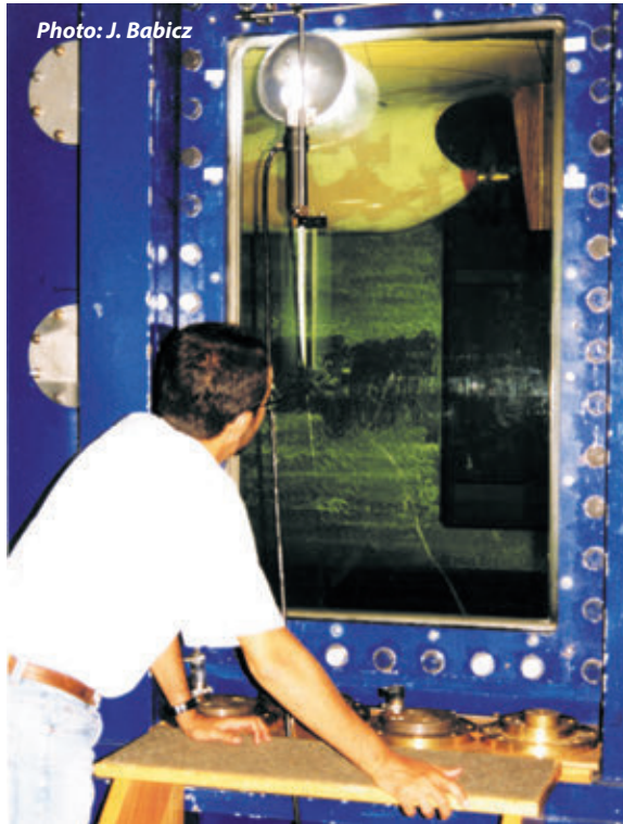
Cavitation test in HYKAT
