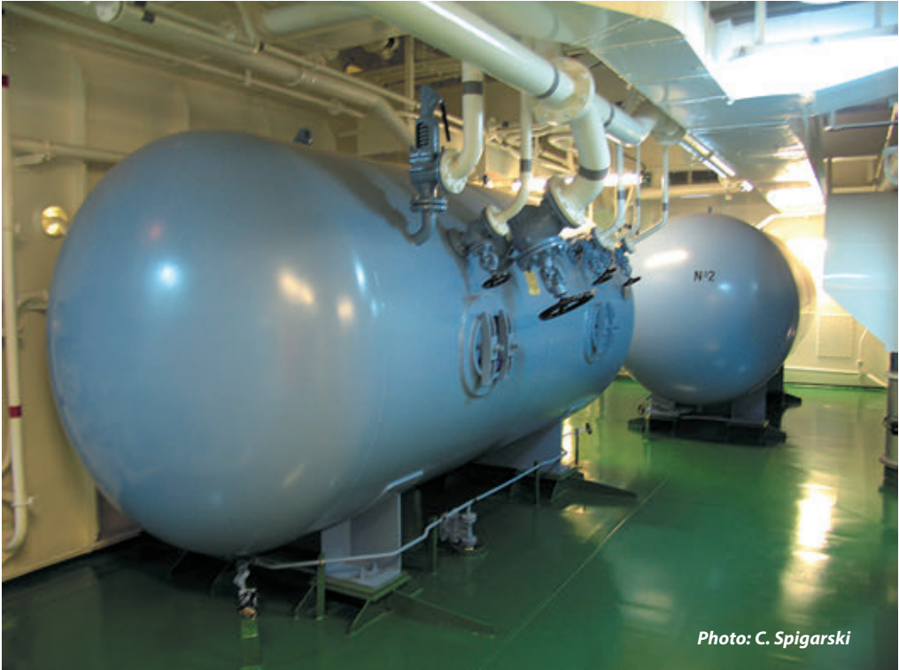
Air receivers onboard the 4444 TEU container vessel MSC FLORIDA designed and built by Gdynia Shipyard
