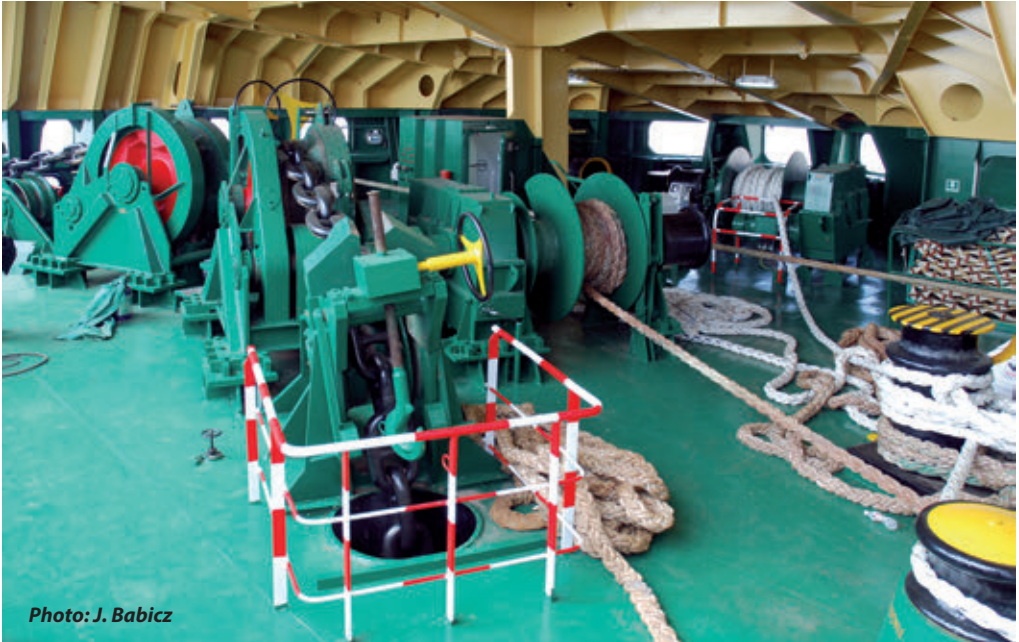
Anchor/mooring equipment on the forecastle deck of 5300 TEU vessel
