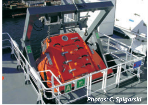
Free-fall lifeboat and launching ramp with integral recovery system onboard car carrier
