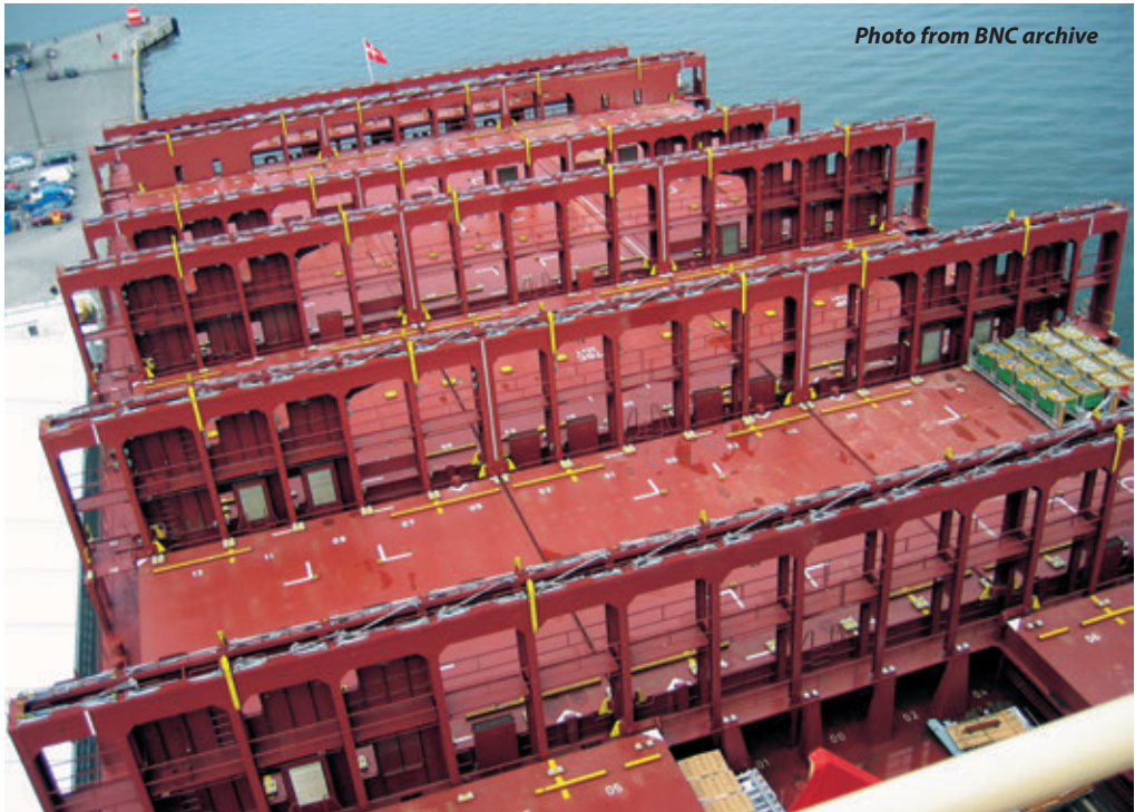
Lashing bridges on an ultra large container vessel
