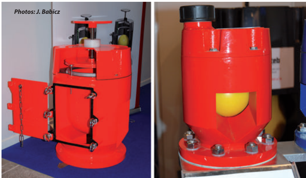
Light, compact air pipe heads from WINTEB enable tank flushing (left) or tank sounding (right)
