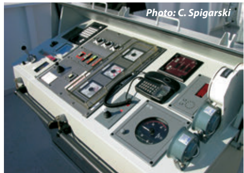
Wrong wheelhouse arrangement with high equipment located in field of vision
