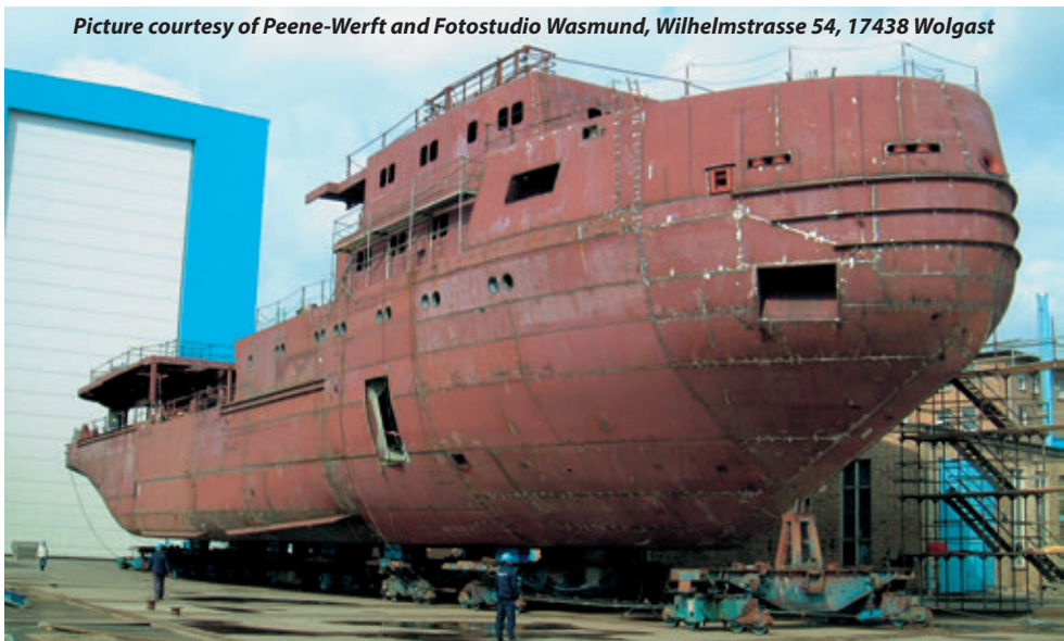
Hull of the oil spill response vessel ARKONA built by PEENE-WERFT (note the icebreaking bow with anchor pocket)
