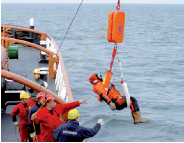
Rescue lifting system with double loop and stopper block
