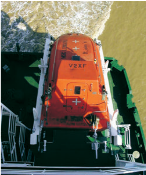
Free-fall lifeboat and simple launching ramp. Recovery by a combined life-saving/provisions crane
