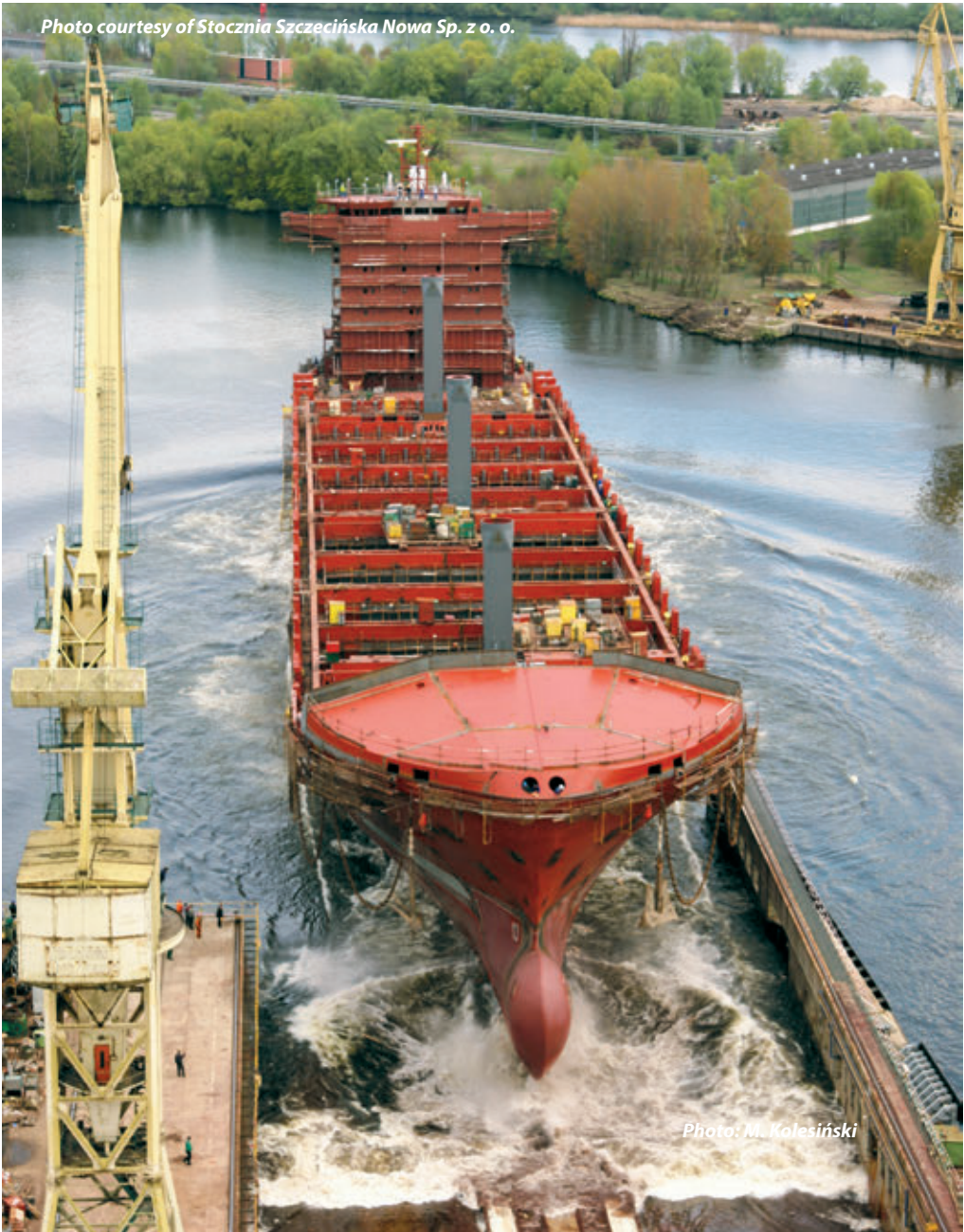
End launching in Szczecin New Shipyard
