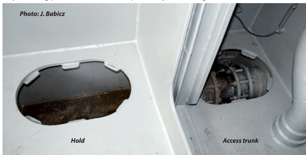
Always accessible bilge well designed by BNC
