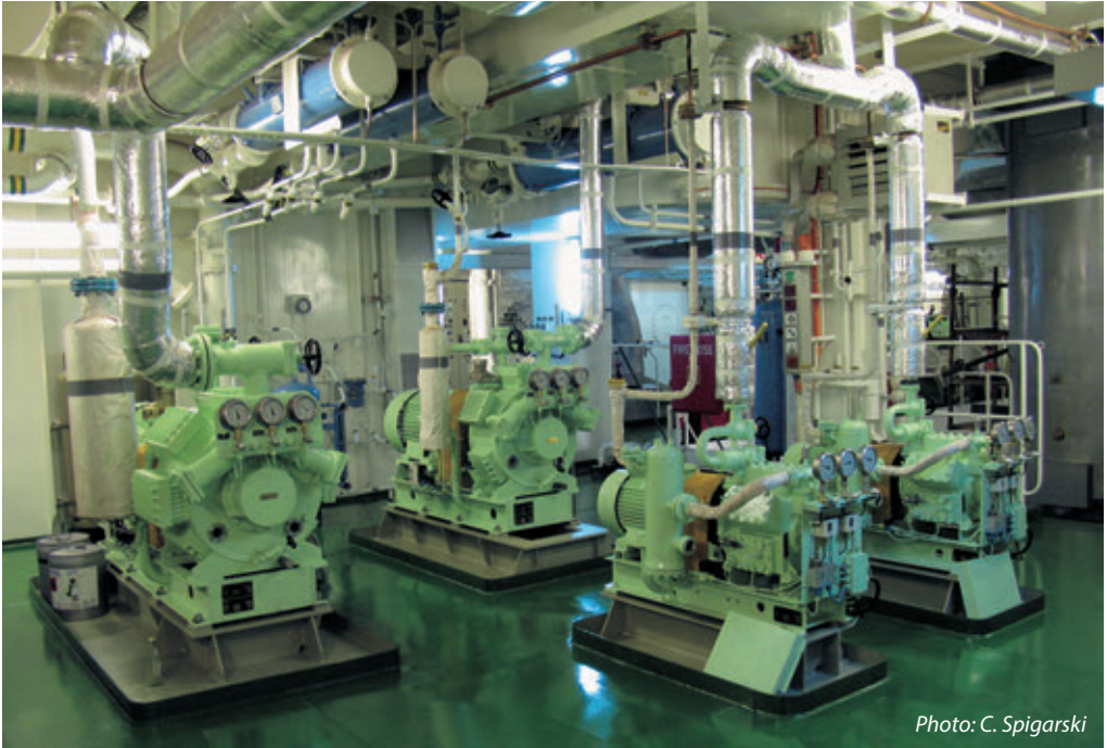
Air compressors onboard the 4444 TEU container vessel MSC FLORIDA built by Gdynia Shipyard
