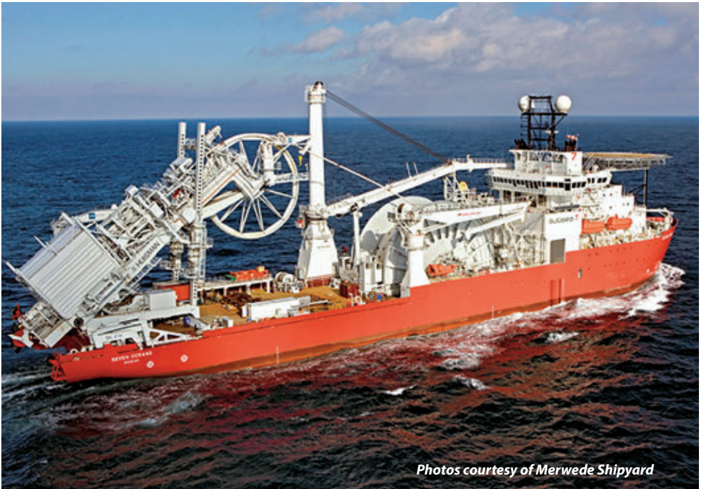
Pipelaying/offshore construction vessel SEVEN OCEANS built by Merwede Shipyard in 2007
