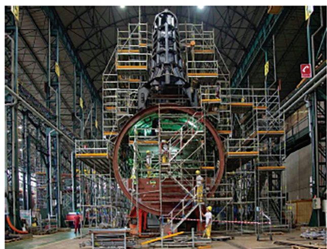
Figure 2: S-80 Isaac Peral-class submarine under construction IMAGE CREDIT: NAVANTIA
