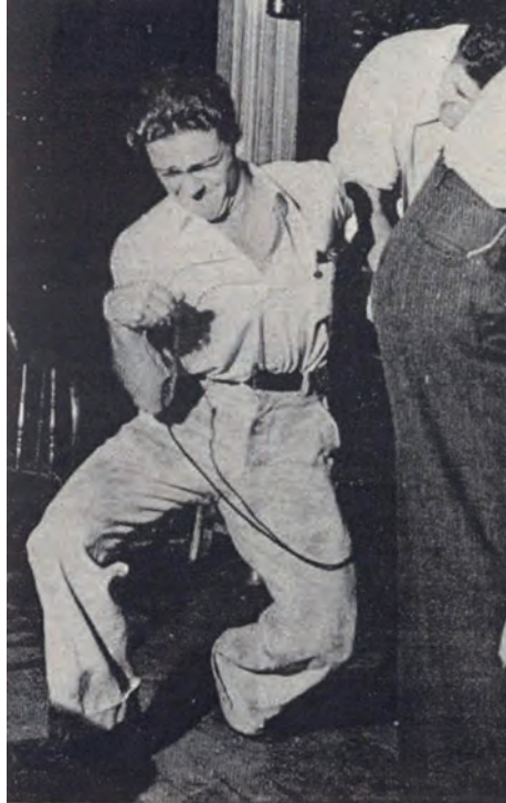
Figure 9.1 A volunteer during secondary electric shock test. (From Charles F. Dalziel, Electric shock hazard , IEEE spectrum, 1972, Courtesy of IEEE.)
