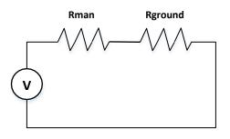
$R_{total} = R_{man} + R_{ground} = 21 \text{ KOhm}$  $I = \frac{V}{R_{total}} = \frac{230}{21000} = 10.95 \text{ mA}$
