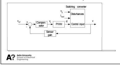
performance can be studied. i<sub>load</sub>(s) H(s)  $=\frac{V_{in}R(1+sCr_c)}{LC(R+r_c)s^2+(RCr_c+RCr_i+Cr_ir_c+L)s+R+r_i}$  $G_{vd}(s) =$  $\frac{DR(1+sCr_c)}{LC(R+r_c)s^2 + (RCr_c + RCr_l + Cr_l r_c + L)s + R + r_l}$  $G_{vg}(s) =$
