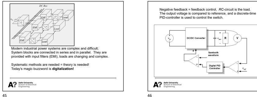
Systems can be described by block diagrams PWM (pulse width modulation) transforms the controller output signal to the duty cycle of the switch; basically that belongs to the operation of the actuator Input voltage.  $V_q$  and load current  $i_{load}$  are disturbances from control viewpoint. Robustness means the ability of the controller to tolerate disturbances and modeling errors.
