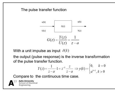
In the inverse transformation similar ideas as in the continuous time case are applied (dividing terms into sums of smaller entities and then using tables)
