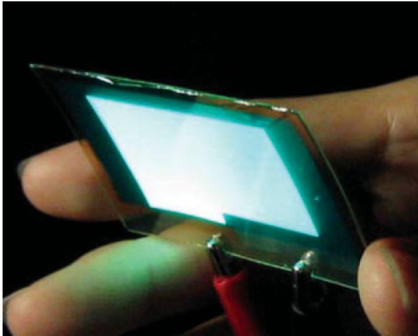
Figure 1. Luminescence of an organic light-emitting diode deposited onto a transparent BC nanocomposite. The luminescence area is 40 \times 25 \text{ mm}^2 . This work was carried out in collaboration with Mitsubishi Chemical Corporation and Pioneer Corporation.
