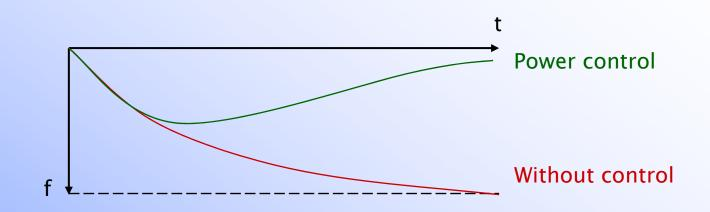
The characteristics of the power controller (droop):
