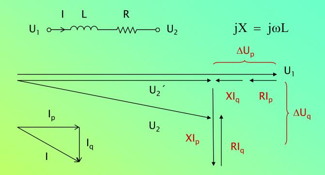
Longitudinal component :  $\Delta U_p = RI_p + XI_q$ Transverse component :  $\Delta U_q = RI_q + XI_p$ For small small  $\Delta U$  (< 10%)
