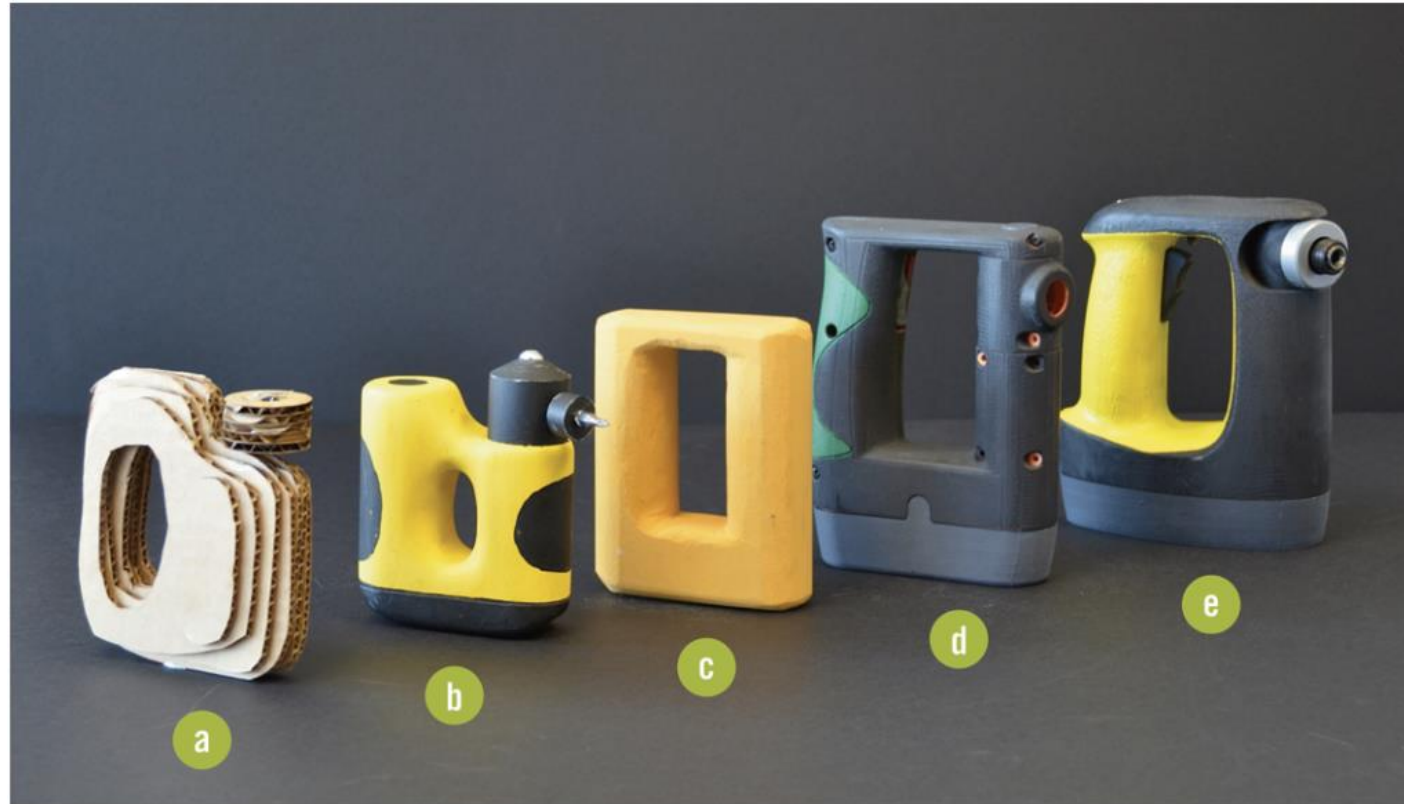
Product development prototypes for cabinet maker's impact driver. The swivel head allows the driver to get into tight spots. (a) Cardboard. (b) Wood. (c) Foam. (d-e) Fused deposition modeling rapid prototypes.
