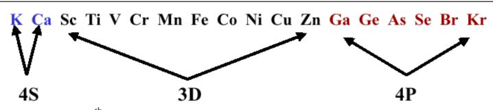
Figure 1. The 4<sup>th</sup> row of the periodic table. The transition metals are the elements that range from Sc (Scandium) to Zn (Zinc).
