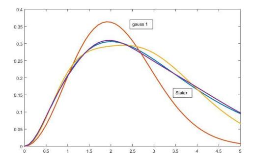
Even an atom might be well described with very few Slater functions (minimal basis set) a reliable description of molecules needs larger basis. Typically, higher angular momentums than the valence electrons have are needed, e.q. dorbital for C, O, N etc. and p-orbitals for H. We need two (or more) exponents since in the molecule the wave functions decay from the nucleus is not symmetric.
