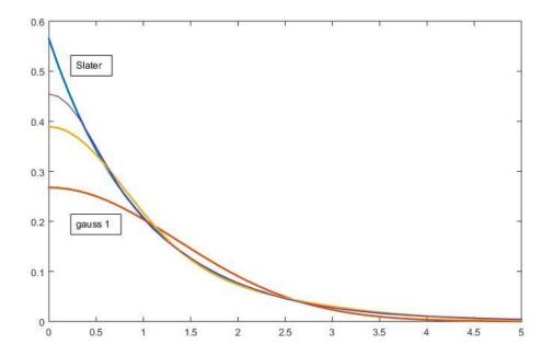
It is also difficult to fit the Slater function at larger distances. Below is the  $r^2\xi_{1s}(r)$  orbitals plotted
