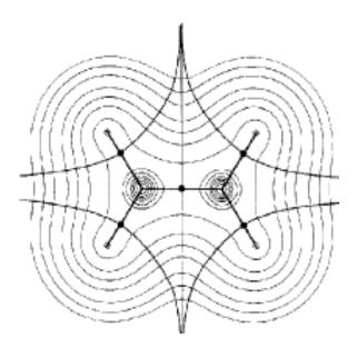
The charges can also be determined from the electrostatic potential. We can find the atomic charges that reproduced best the total el. potential.
