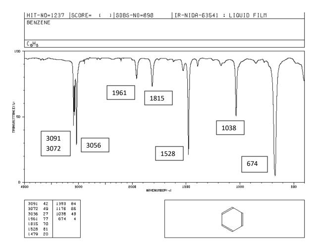
above is the IR spectra (PBE, TZVP, DFT-GGA model, with def2-QZVPP basis gave 2-6 cm<sup>-1</sup> smaller freq) of benzene and below the computed frequencies. See the PBE0 values in the boxes. Check the agreement. Is something missing? -----
