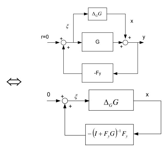
The "Small gain theorem" guarantees that the closed loop is stable, if subsystems are stable and the gain of their product
