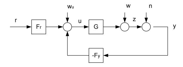
The system is internally stable, if (after all cancellations in the calculation of the transfer functions have been made) the following transfer functions
