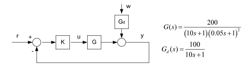
Command tracking + disturbance rejection problem Both demands are difficult to meet simultaneously (trade-off in control design)
