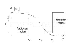
The change should be fast (as S must grow, let it happen fast in a small frequency range, in order to force T to be small).
