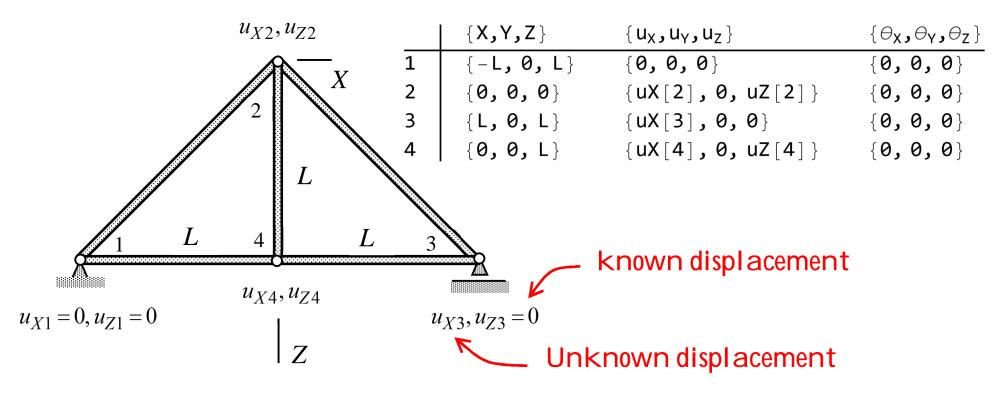
If the value of a nodal displacement or rotation is known, the value is used instead of a symbol in the table!
