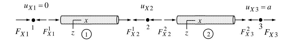
• As the axes of the structural and material coordinate systems coincide in this case so for element 1  $F_{x1}^1 = F_{X1}^1$ ,  $F_{x2}^1 = F_{X2}^1$ ,  $u_{x1}^1 = u_{x1} = 0$ ,  $u_{x2}^1 = u_{x2}$  and for element 2  $F_{x2}^2 = F_{x2}^2$ ,  $F_{x3}^2 = F_{x3}^2$ ,  $u_{x2}^2 = u_{x2}$ , and  $u_{x3}^2 = u_{x3} = a$ . In terms of the force and displacement
