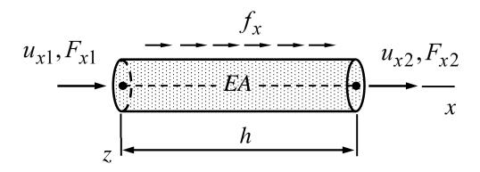
force-displacement relationship of a bar element!
