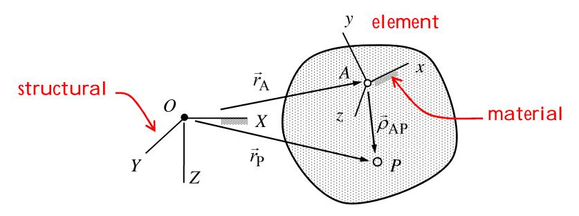
The basis vectors of the material and structural systems are denoted by  $\vec{i}$ ,  $\vec{j}$ ,  $\vec{k}$  and  $\vec{l}$ ,  $\vec{J}$ ,  $\vec{K}$ , respectively!
