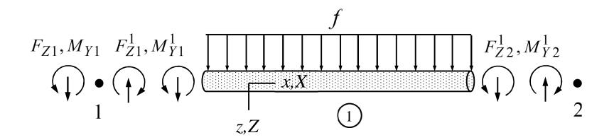
• Element contribution, when the known displacement and rotation at the left end  $u_{Z1} = \theta_{Y1} = 0$  are substituted there, and the equilibrium equations of nodes 1 and 2:
