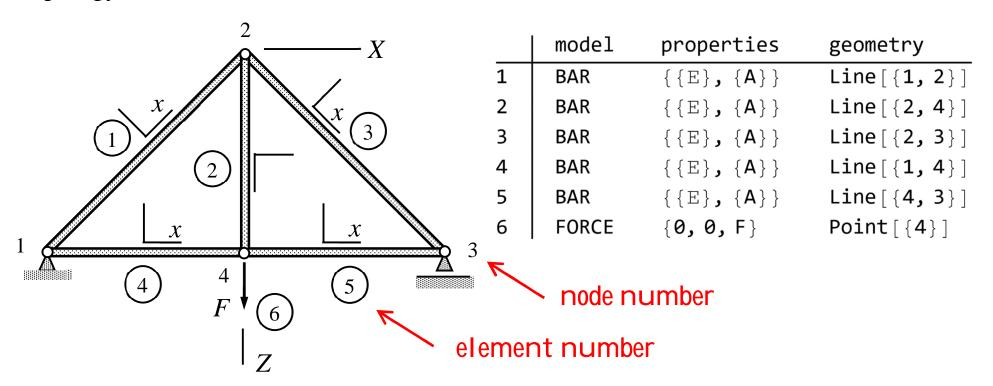
The order of the nodal numbers in the table depends on the orientation of the elementwise material coordinate systems.
