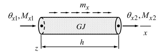
the force-displacement relationship of torsion bar element!
