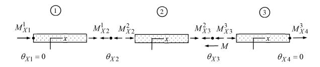
Element contributions of the torsion bar elements 1, 2 and 3 (formulae collection) and the equilibrium equations of nodes 2 and 3 are (notice that the distributed moment vanishes here)
