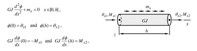
in which the shear modulus G, cross-sectional area of the bar A, and external distributed moment per unit length  $m_x$  are constants. Derive the element contribution of a torsion bar element with the aid of the boundary value problem.
