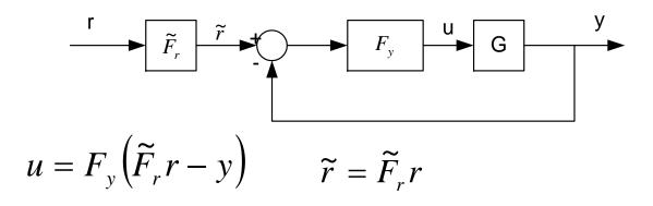
A two-degrees-of-freedom structure can be interpreted as a one-degree-of-freedom structure, in which the reference signal has been filtered by a prerefilter.
