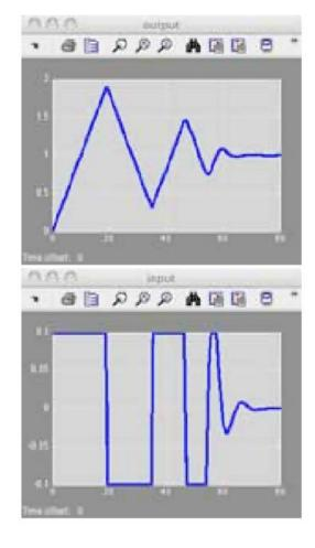
very simple process (=an integrator) controlled by a PID controller ( $K_P = K_I = K_D = 1$ ) under saturation  $-0.1 \le u \le 0.1$
