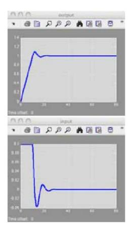
anti-windup scheme for a PID controller ( $K_P = K_I = K_D = 1$ ,  $T_t = 1$ )
